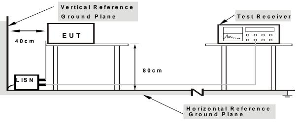
Note: 1.Support units were connected to second LISN. 2.Both of LISNs (AMN) are 80 cm from EUT and at least 80
