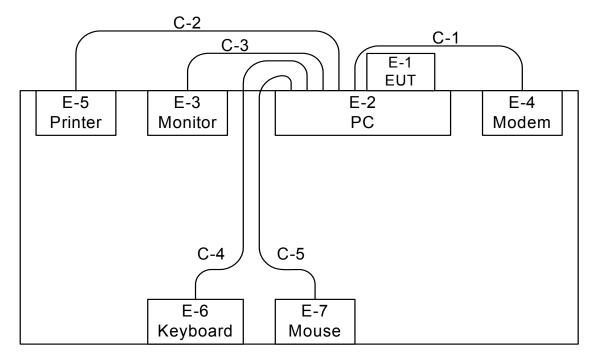
C-1: RS232 Cable C-2: Parallel Cable C-3: D-Sub Cable C-4: USB Cable C-5: USB Cable
