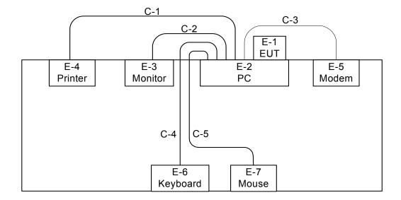
C-1: Parallel Cable C-2: D-Sub Cable C-3: RS232 Cable C-4: USB Cable C-5: USB Cable
