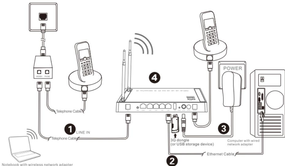
2.1. Connect the DSL line with the attached telephone cable.
