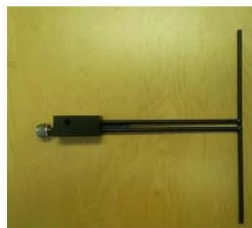
Figure 1 – MVG COMOSAR Validation Dipole
