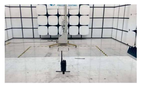
RADIATED EMISSION TEST SETUP
