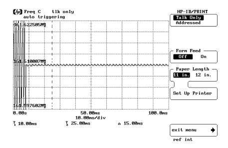
Transmitter Frequency Behavior @ 12.5 KHz Channel Separation--On to Off-10W
