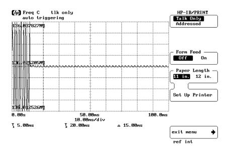
Transmitter Frequency Behavior @ 12.5 KHz Channel Separation--On to Off
