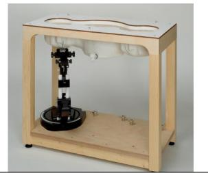
The bottom plate contains three pair of bolts for locking the device holder. The device holder positions are adjusted to the standard measurement positions in the three sections. A white cover is provided to tap the phantom during off-periods to prevent water evaporation and changes in the liquid parameters. On the phantom top, three reference markers are provided to identify the phantom position with respect to the robot.
