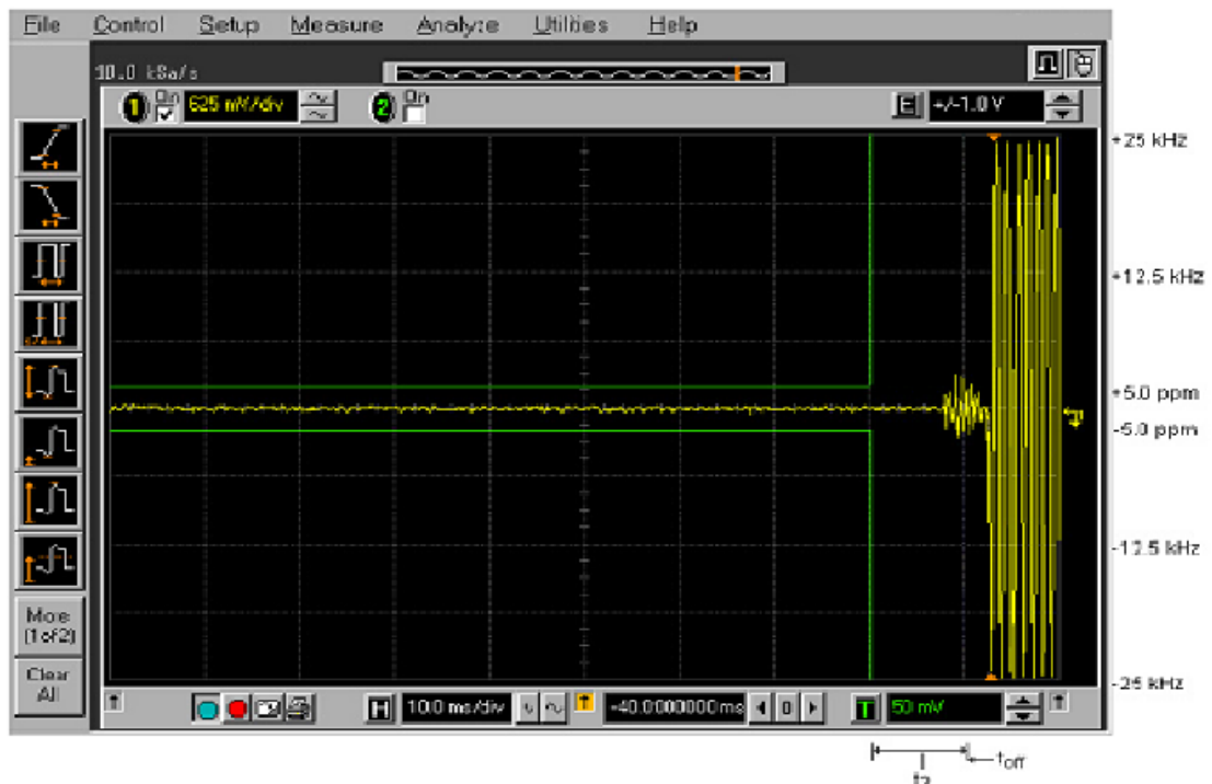
Transmitter Frequency Behaviour @ 12.5 KHz Channel Separation--On to Off
