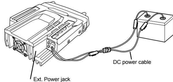
optional QCC-01(For Cigar-Plug connection) cable. Connect one of the cables between the ACC terminal or a Cigar-Plug that operates with the vehicle ignition or ACC switch on the vehicle and EXT POWER jack on the rear side of the unit.
