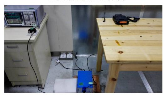
RADIATED EMISSION TEST SETUP BELOW 1GHz
