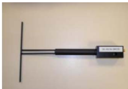
Figure 1 – Satimo COMOSAR Validation Dipole
