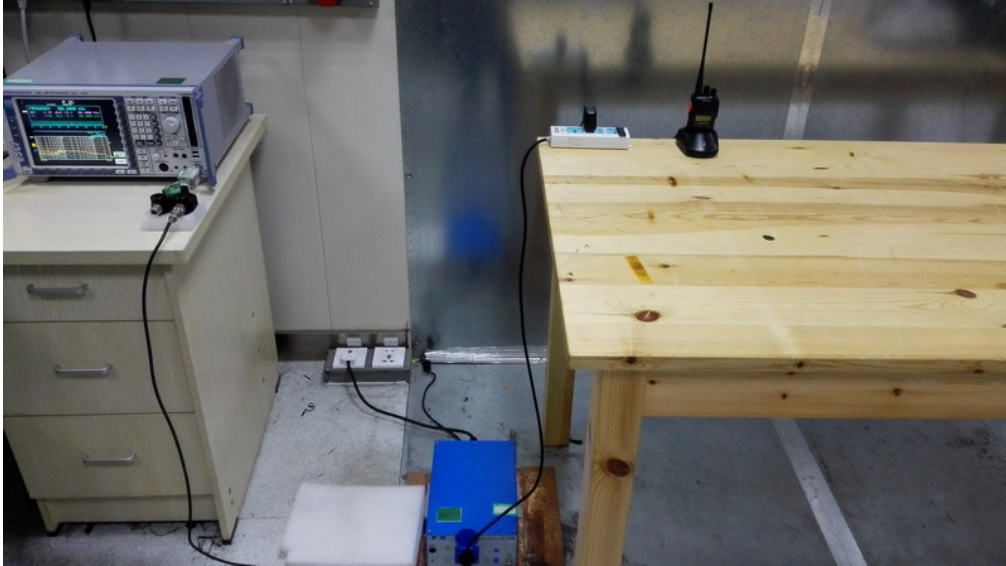
RADIATED EMISSION BELOW 1GHz TEST SETUP
