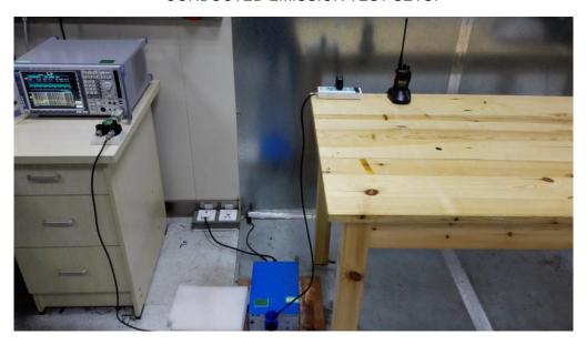
RADIATED EMISSION BELOW 1GHz TEST SETUP
