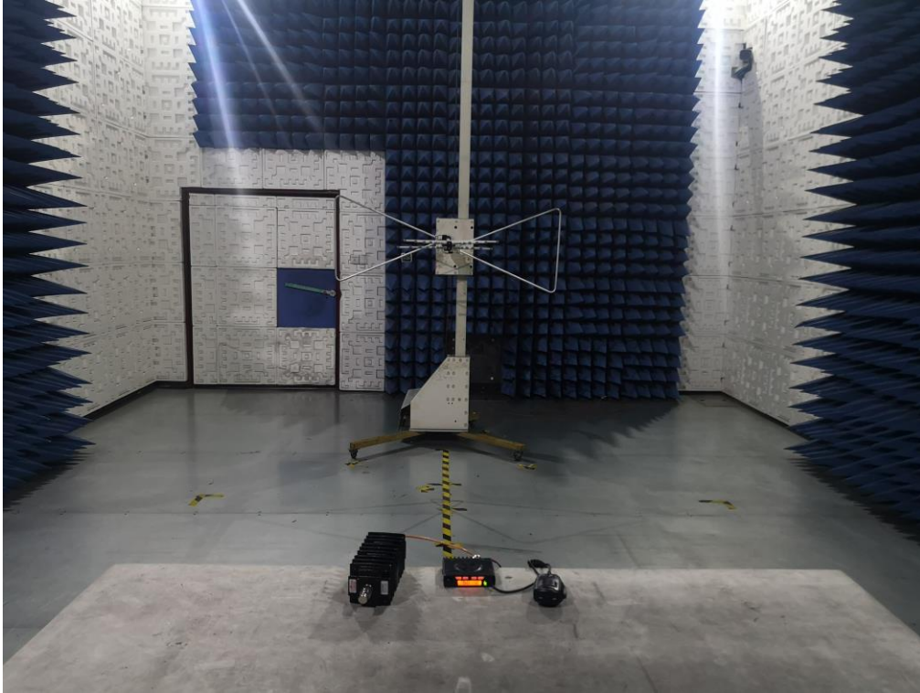
RADIATED EMISSION TEST SETUP-ABOVE 1GHZ
