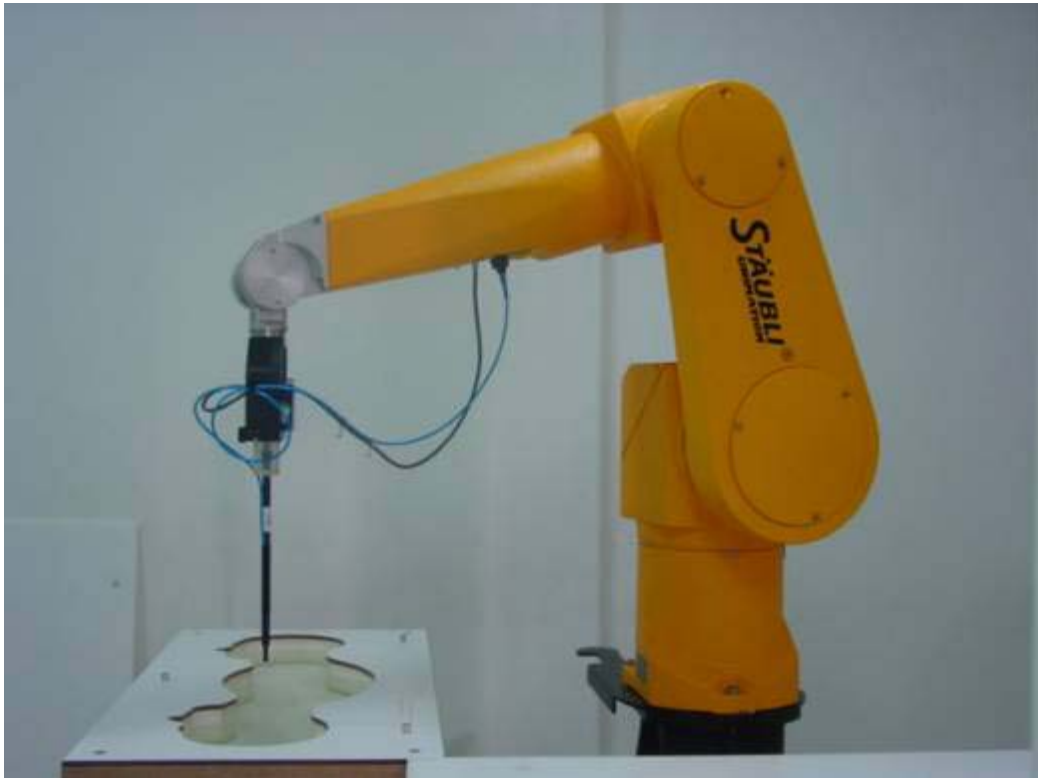
Picture 1: Specific Absorption Rate Test Layout
