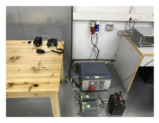
RADIATED EMISSION TEST SETUP-BELOW 1GHz
