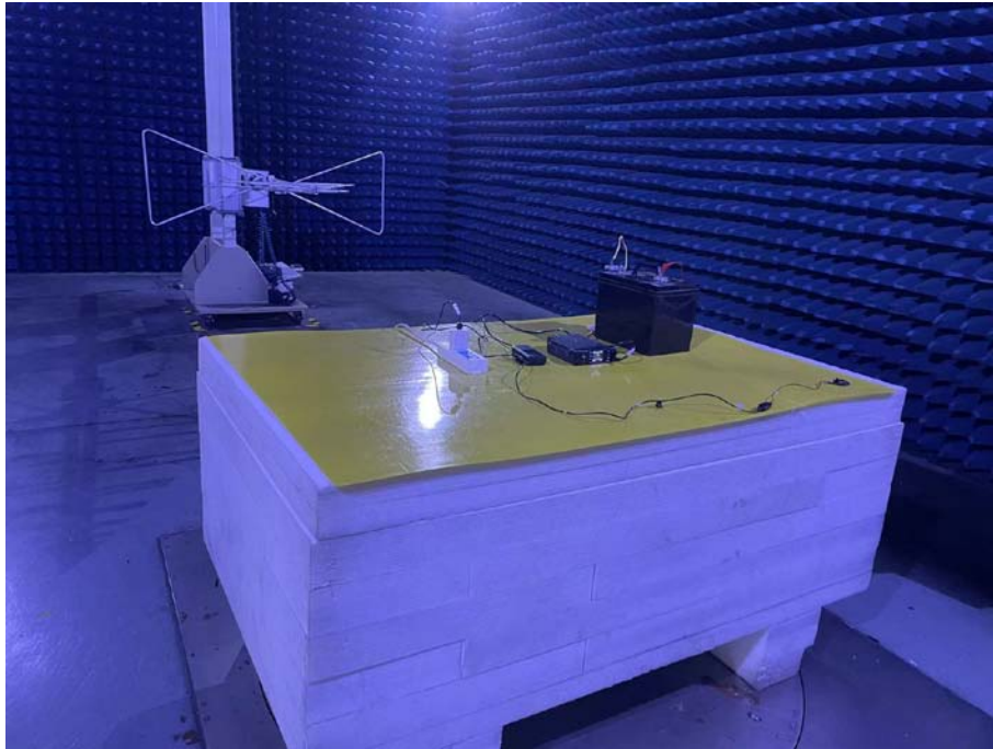
Photo of Radiated Emission Measurement Below 1GHz
