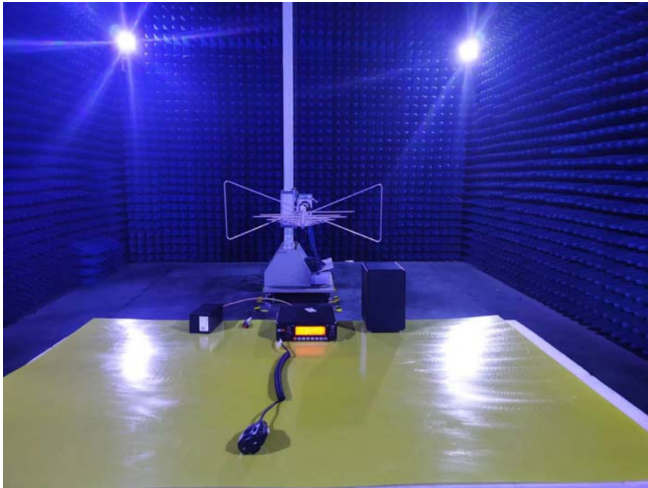
Photo of Radiated Emission Measurement (Below 1G)
