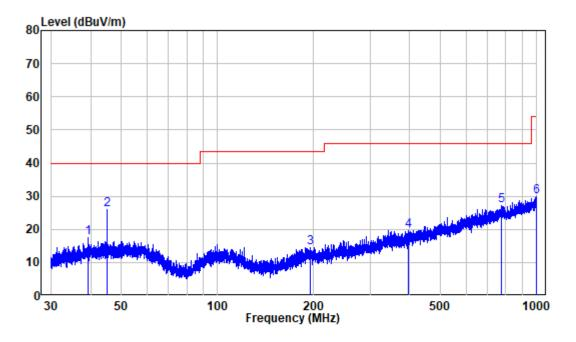
Site : chamber Condition: 3m VERTICAL Job No. : XMTN1220117-02447E-EM Test Mode: scan(receiver)
