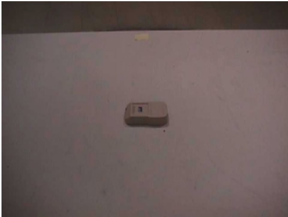
FCC 30-1,000MHz RADIATED EMISSIONS TEST CONFIGURATION TEMPERATURE/HUMIDITY SENSOR 5m SEMIANECHOIC CHAMBER LEXMARK INTERNATIONAL, LEXINGTON KY.
