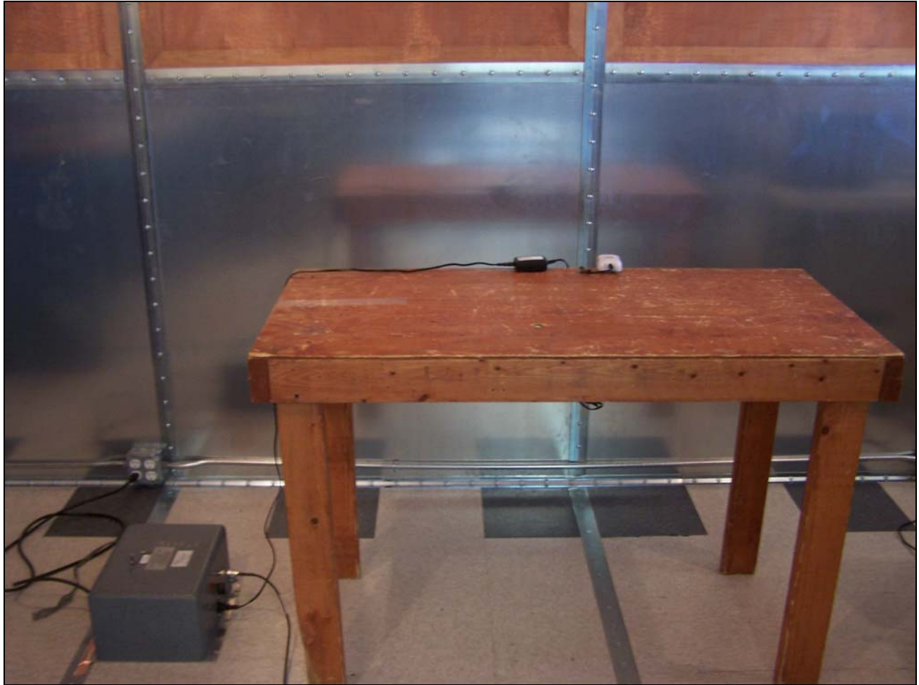
Photograph 5. Conducted Emissions Test Setup
