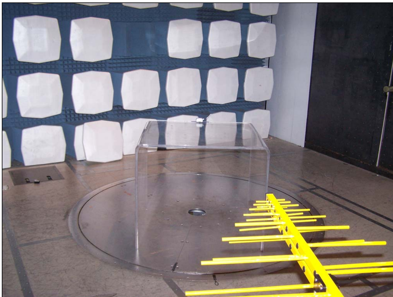
Photograph 2. 15.109, Subpart B Radiated Emissions Test Setup, Normal Operation
