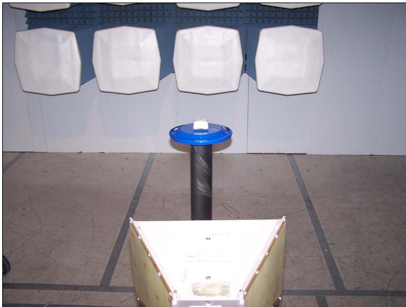
Photograph 4. Spurious Radiated Emission Test Setup
