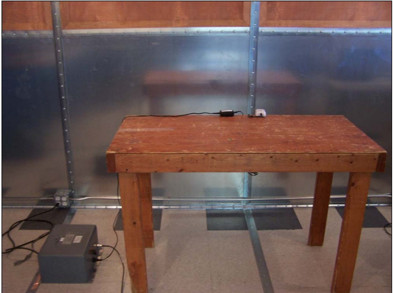
Photograph 1. 15.107, Subpart B Conducted Emissions Test Setup
