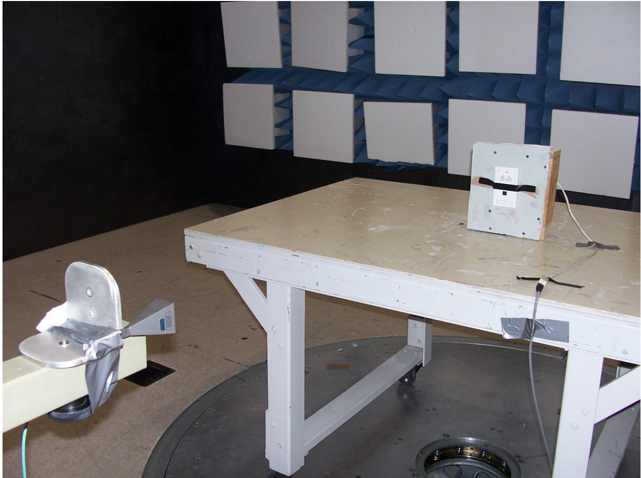
Figure 5 - Radiated Emissions Test Setup (26 - 40 GHz shown)
