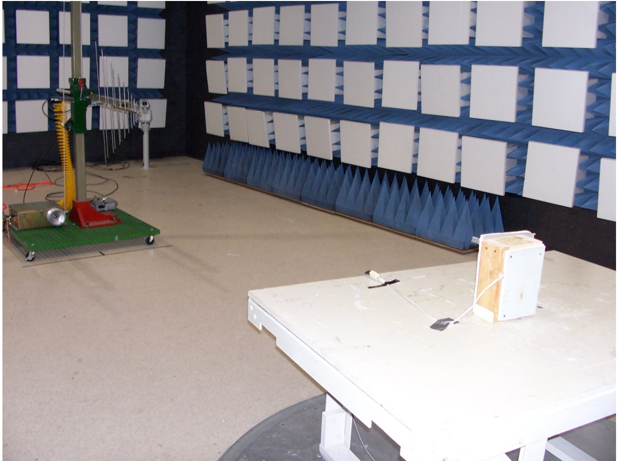
Figure 2 - Radiated Emissions Test Setup (200 – 1000 MHz shown)
