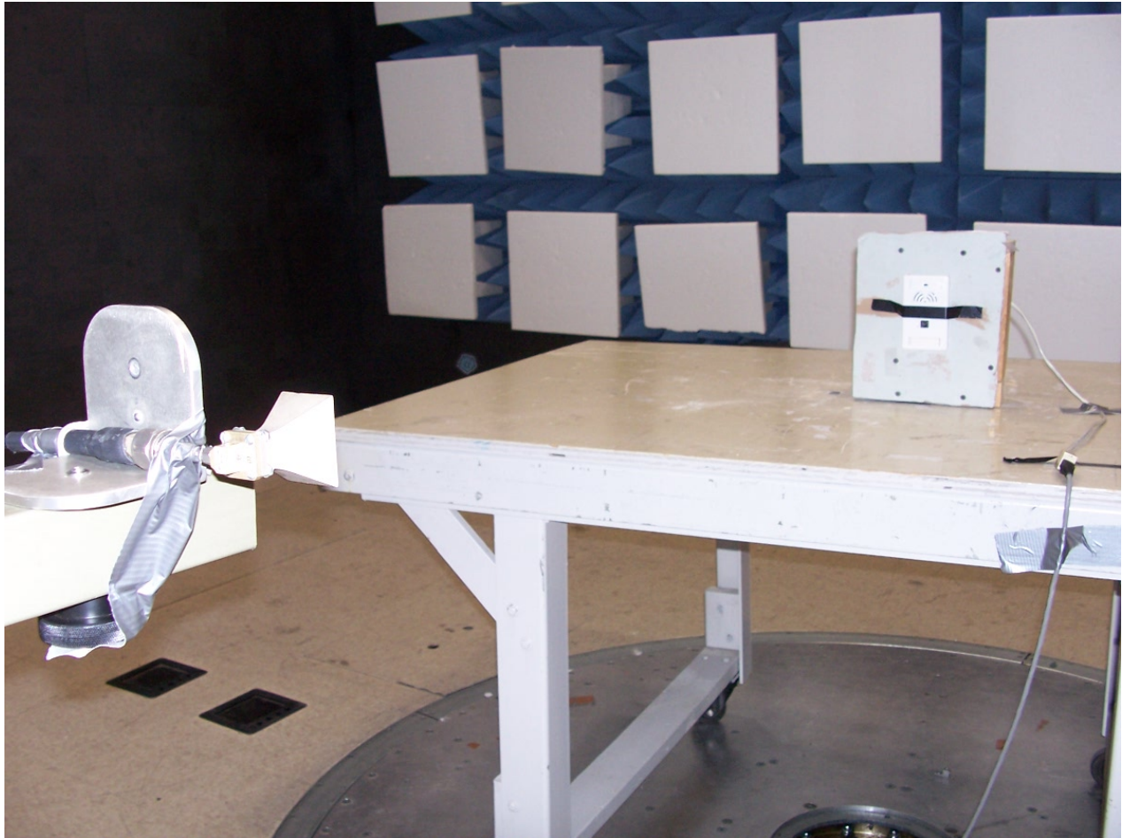
Figure 4 - Radiated Emissions Test Setup (18 - 26 GHz shown)
