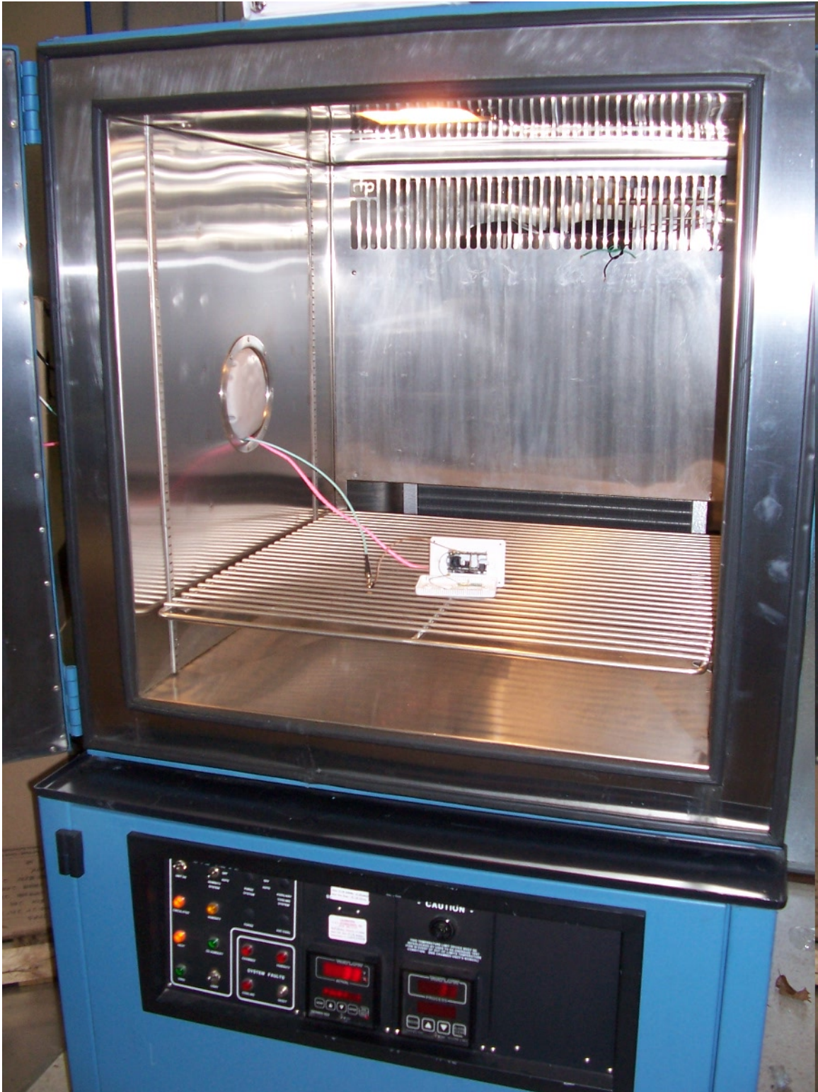
Figure 10 – Frequency Stability - Temperature test set up
