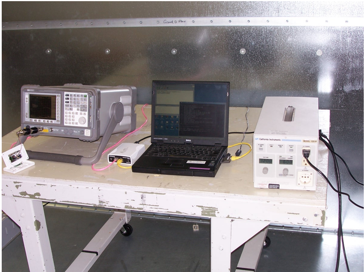
Figure 11 – Frequency Stability – AC Voltage variations
