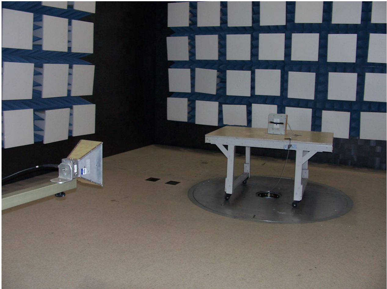
Figure 3 - Radiated Emissions Test Setup (1 – 18 GHz shown)
