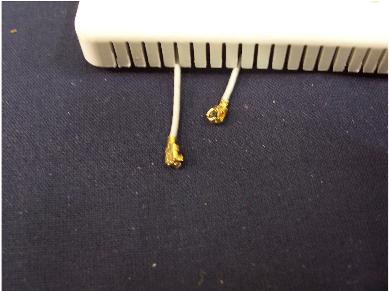
Figure 6 – View of antenna connections on antennas
