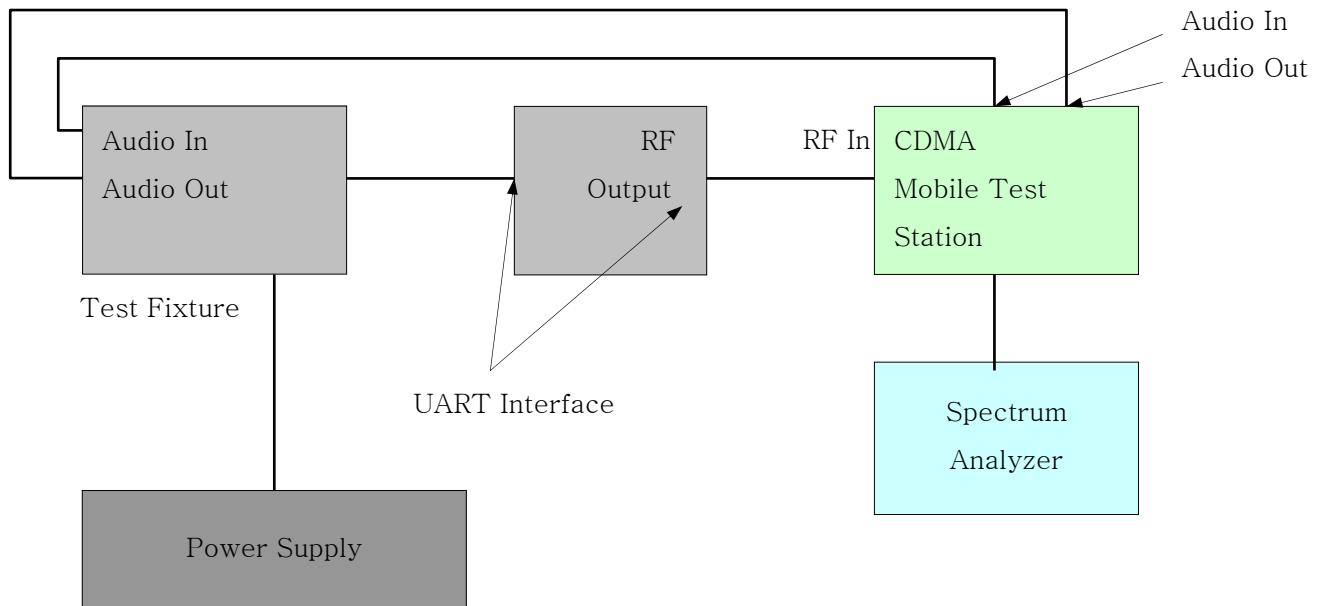
**UART Interface:** The UART Interface has a serial communication link that can be used to test , debug or upgrade the phone's functions and characteristics.
