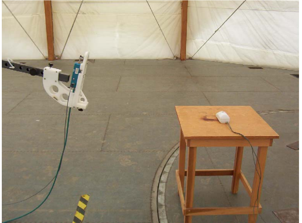
Setup for Spurious emissions on 10 meter OATS – Final test
