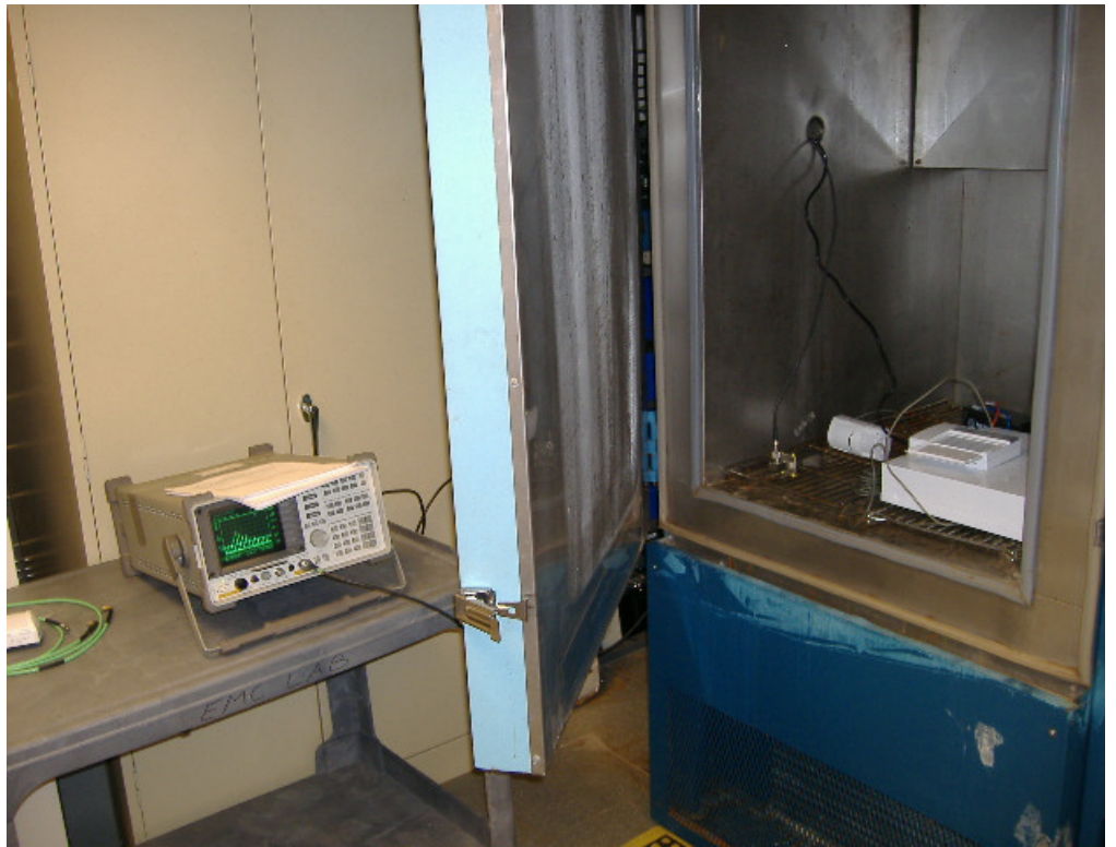
Setup for Frequency Stability over Temperature Variations
