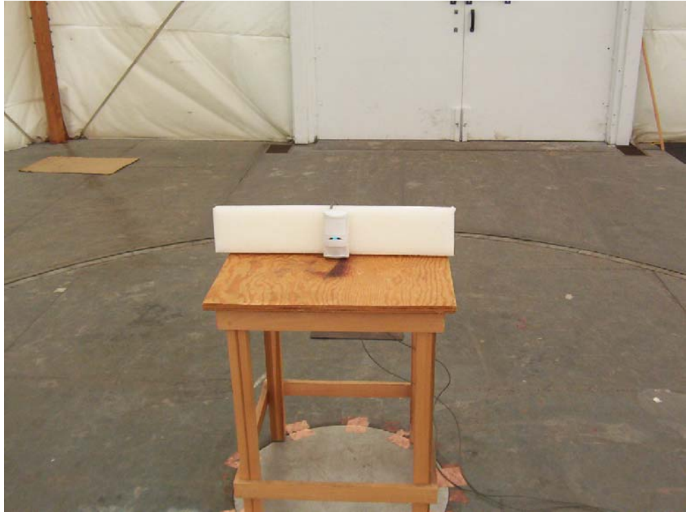
Setup for Radiated emissions on 10 meter OATS – Final test
