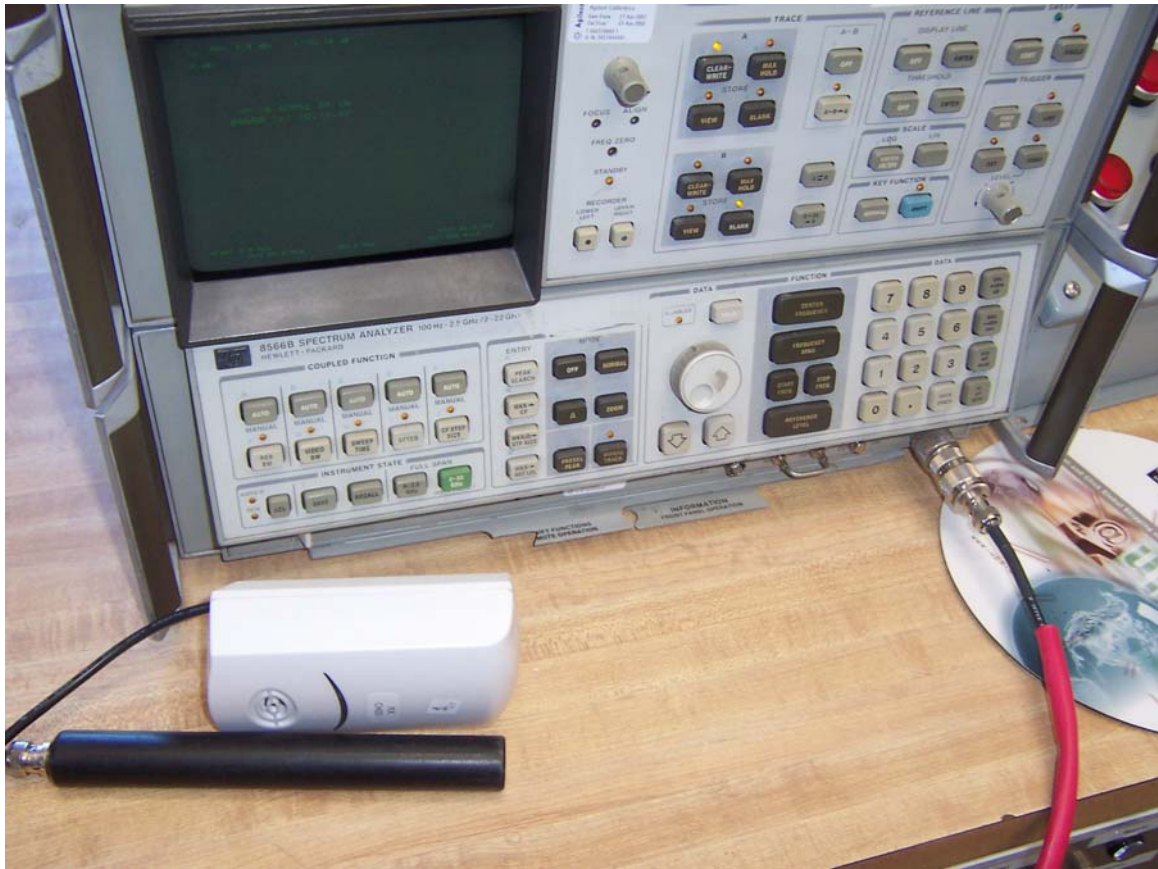
BW, Occupancy Time, 20 dB BW, Carrier frequency separation, Duty cycle Test Setup
