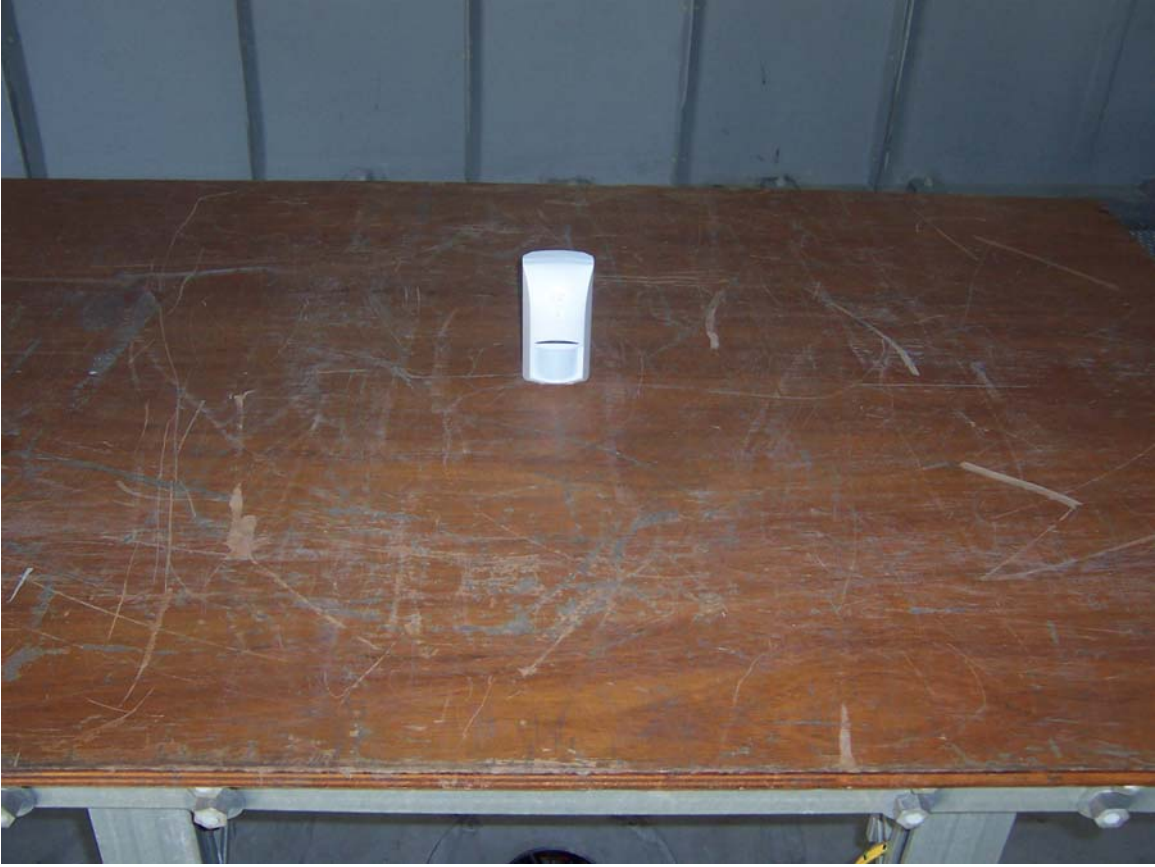
Radiated Emissions Test setup Z-Axis
