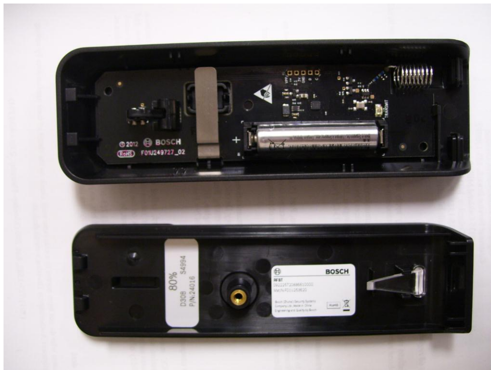
Figure 11: Internal View – RFBT
