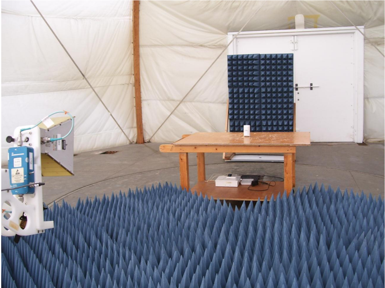
Figure 4: Setup for fundamental and harmonic emissions
