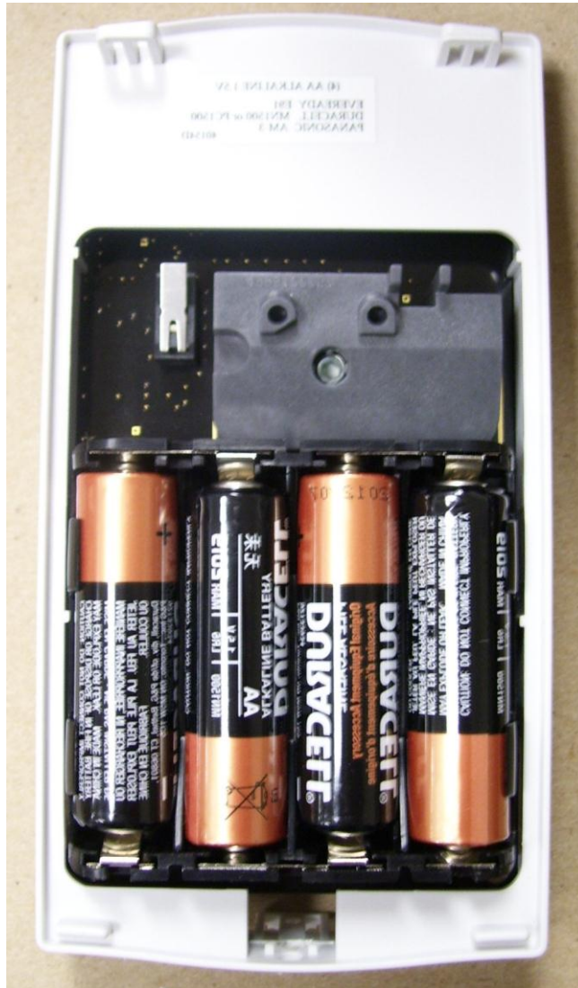
Figure 1: Internal View of Bosch RFDL-11 Sensor Battery cover off
