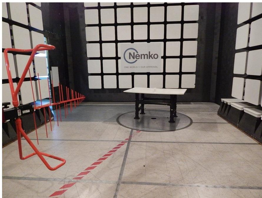
Figure 8.2-1: Radiated emissions setup photo – 30 to 1000 MHz
