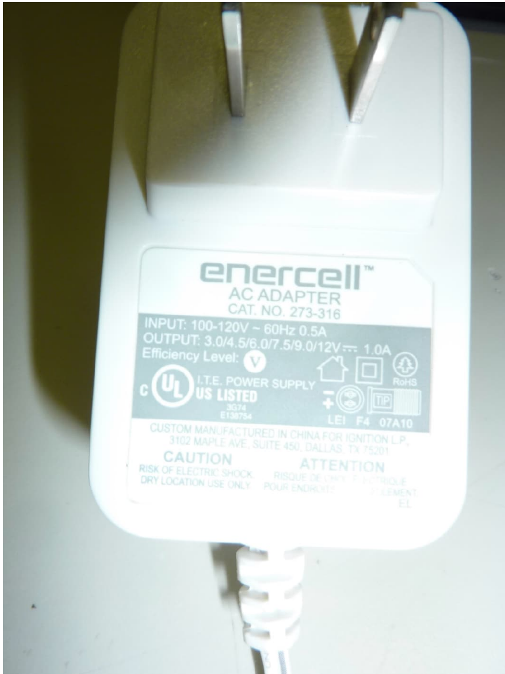
Used AC/DC adaptor for conducted emissions on power supply line
