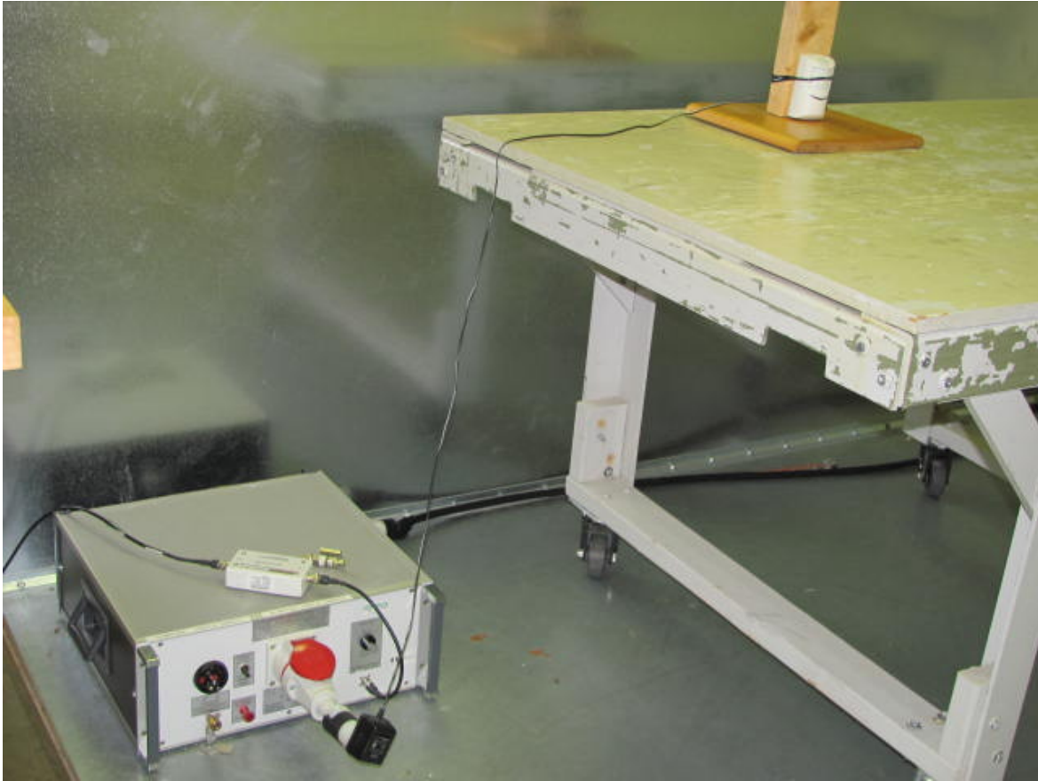
Figure 8: Conducted Emissions on power line.
