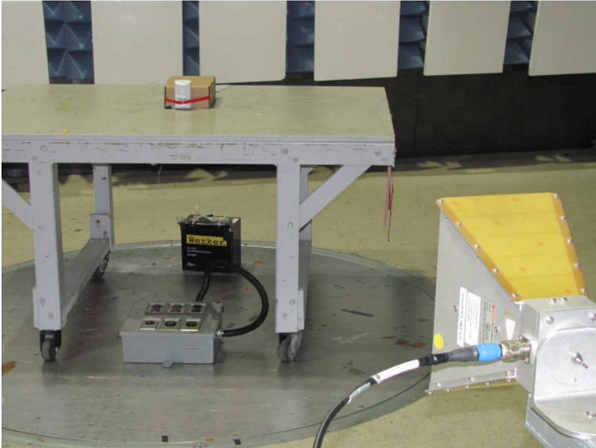
Figure 2: Radiated Emissions at 3m – 1 GHz to 18 GHz.
