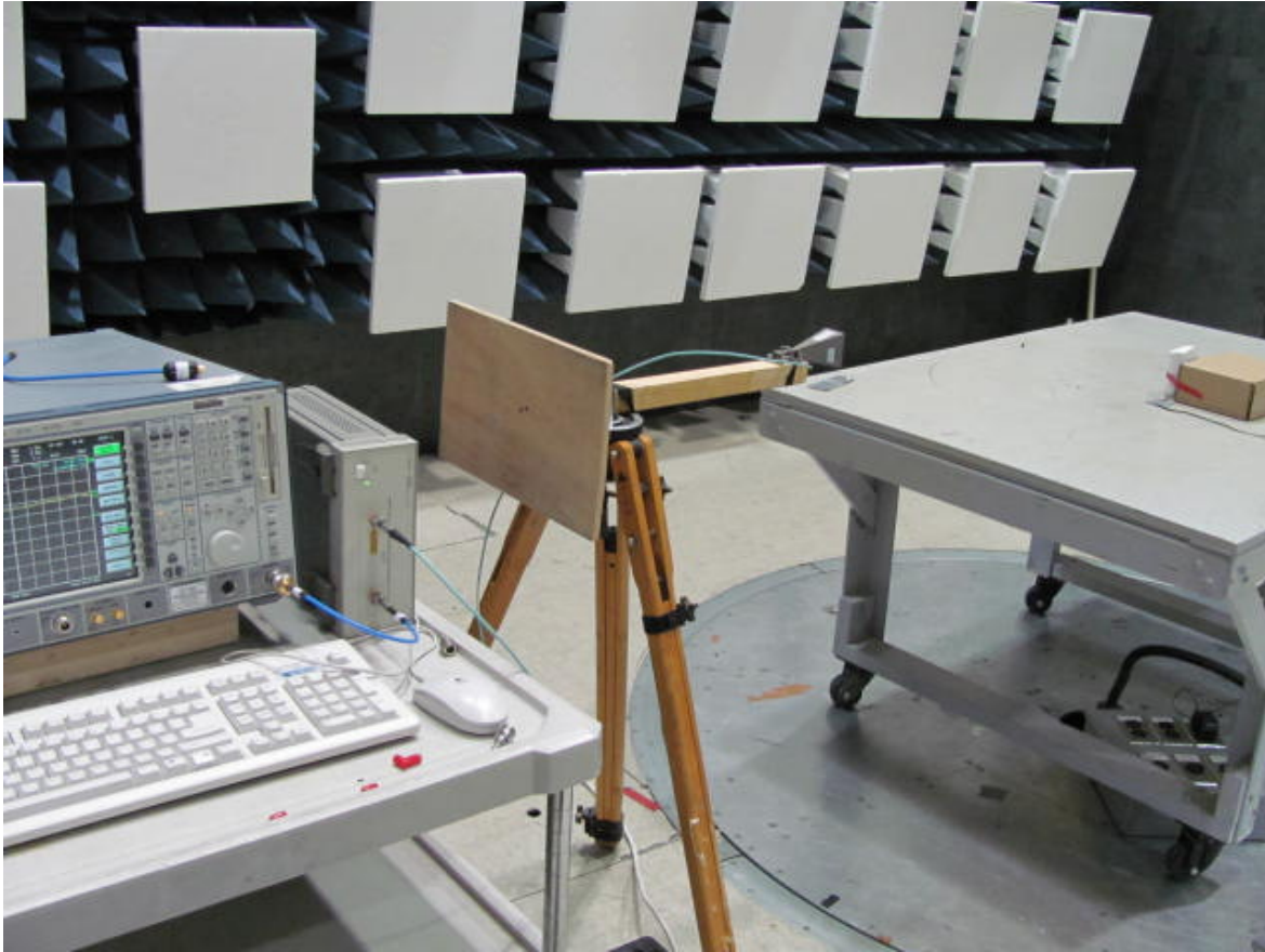
Figure 3: Radiated Emissions at 1m – 18 GHz to 26.5 GHz.
