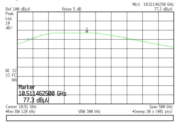
Worst Case: The -20dBc is at 10.50891977GHz which is 8.92 MHz above the band-edge at 10.5 GHz.
