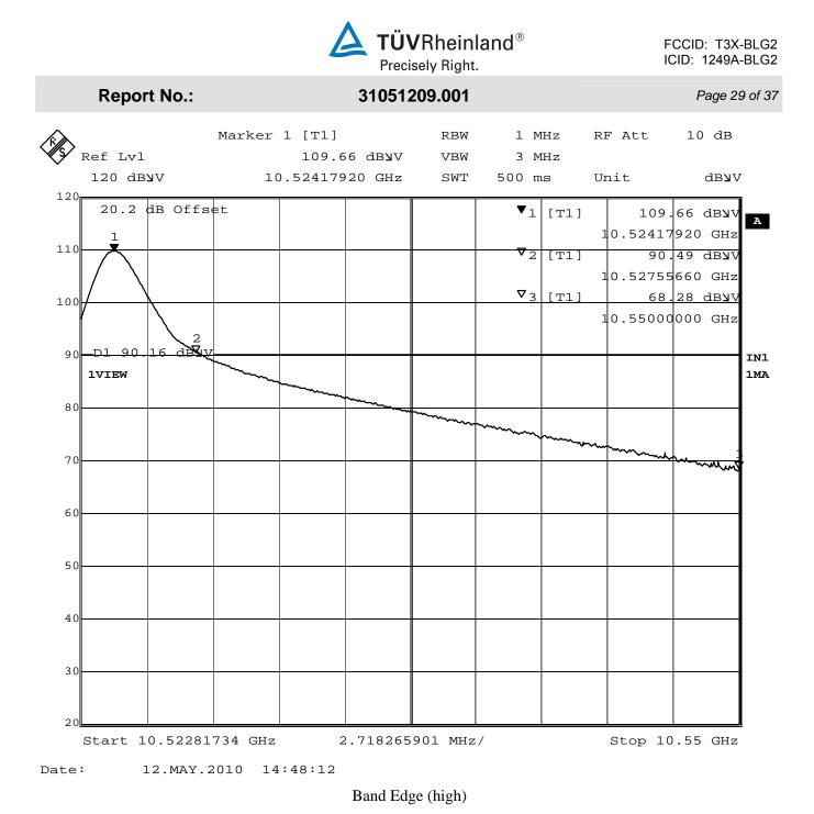
Note: Measurements made using the procedures of ANSI C63.10-2009
