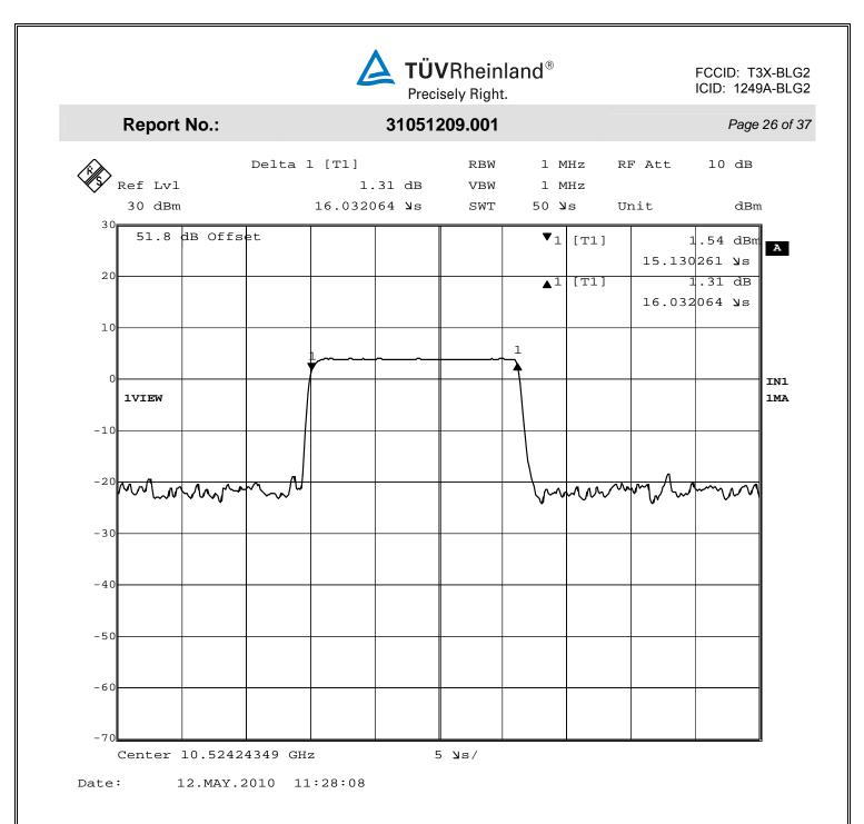
Duty Cycle: Single Pulse = 16.03µs 120 \*16.03µs Pulses = 1.92 ms; 1.92ms / 100 ms = .019or 1.9 %
