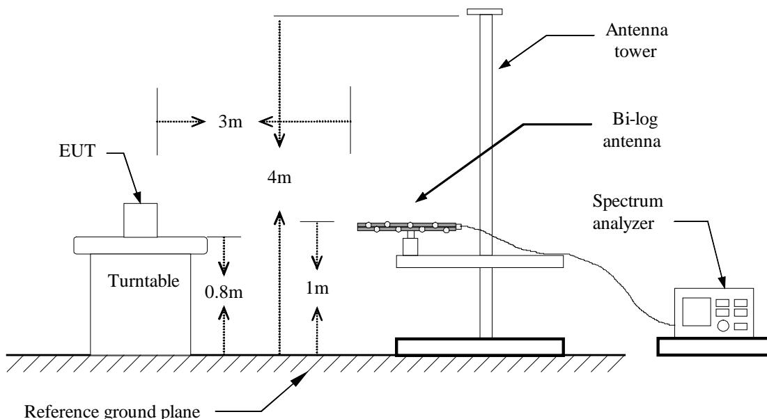
**Above 1 GHz**
