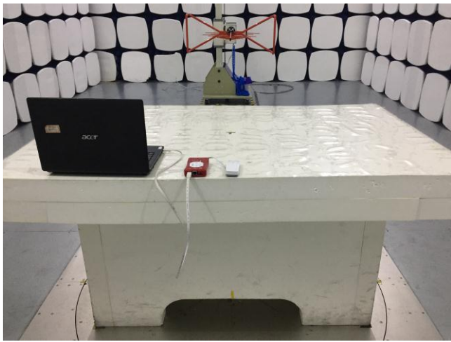
Radiated Spurious Emissions Test Setup Below 1GHz
