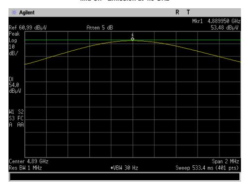
Measurements were taken up to the 10<sup>th</sup> harmonic of the device. No emissions were detected from 18-25 GHz, only noise floor was measured.
