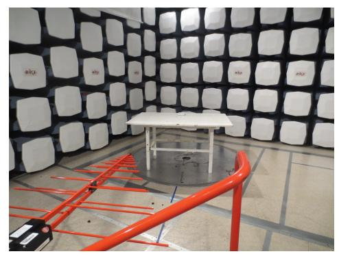
13.2 Radiated Emission below 1 GHz Rear View
