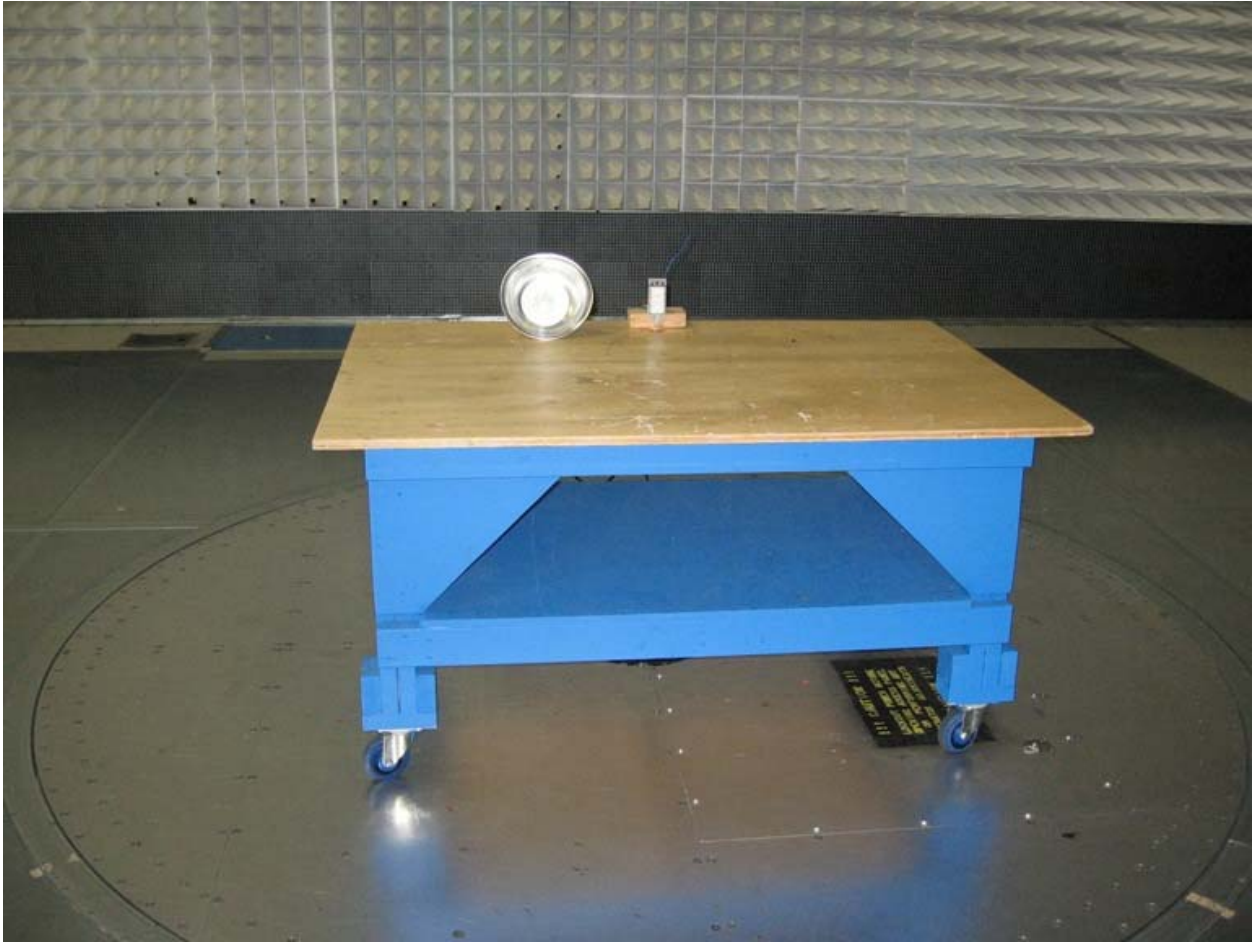
Radiated Emissions – Front View
