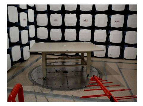
**10.2** Radiated Emissions (Below 1 GHz) – Rear View
