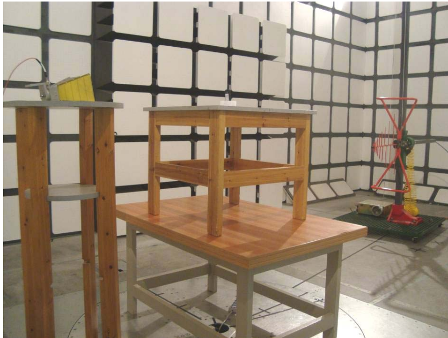
Below 1 GHz: Spurious Radiated Emissions - Rear View
