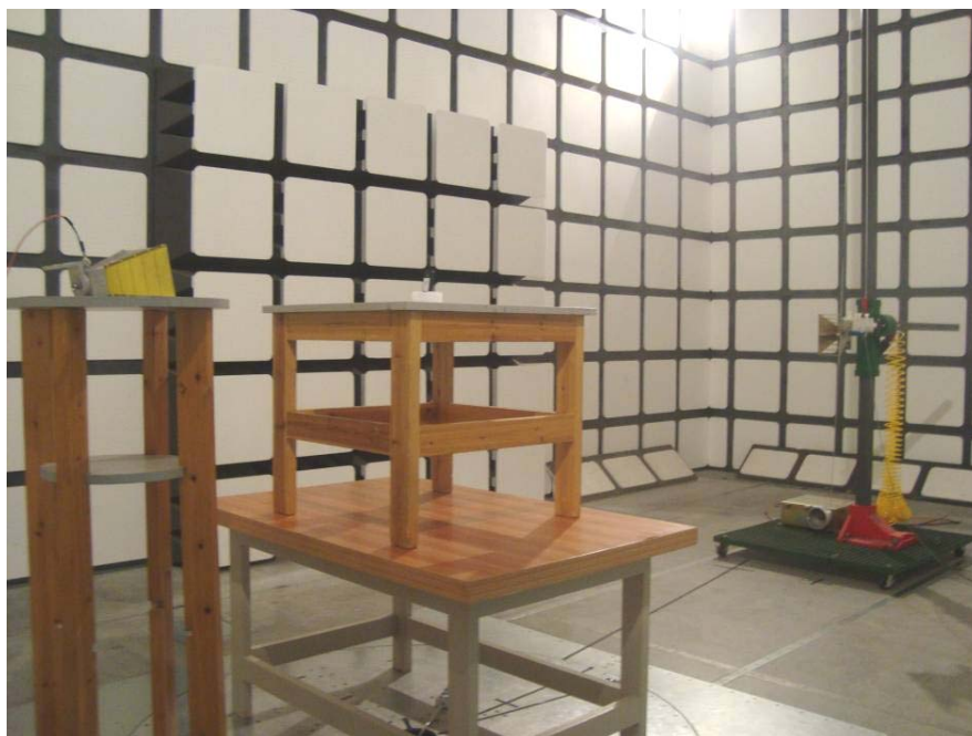
Above 1 GHz: Spurious Radiated Emissions - Rear View
