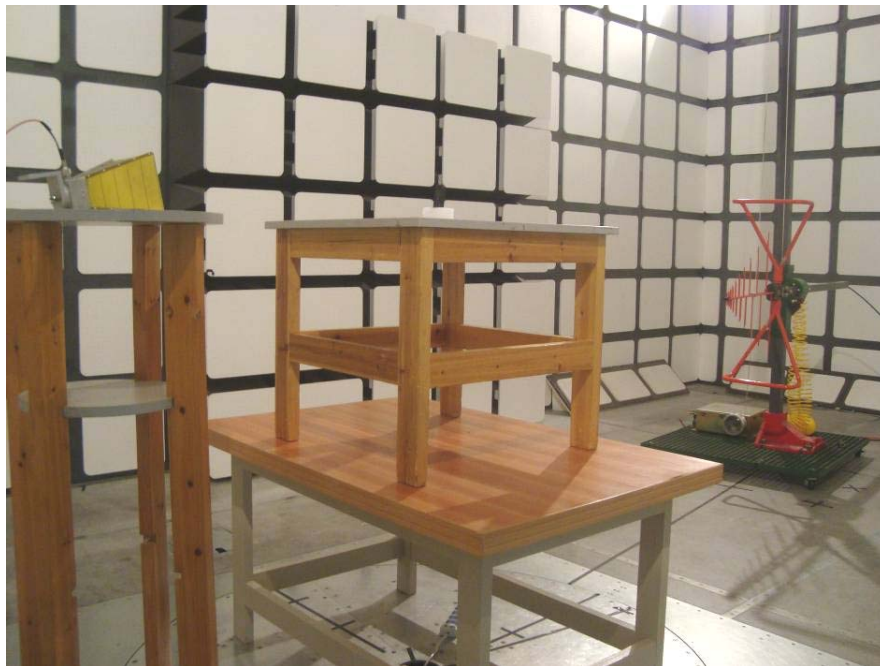
Below 1 GHz: Spurious Radiated Emissions - Rear View
