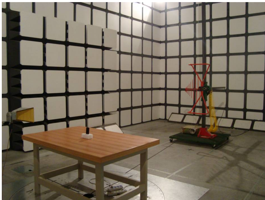
Below 1 GHz: Spurious Radiated Emissions - Rear View
