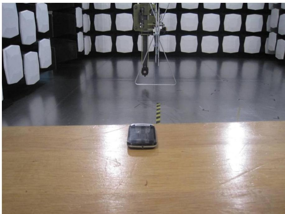
10. Part 15C Radiated emission above 1 GHz
