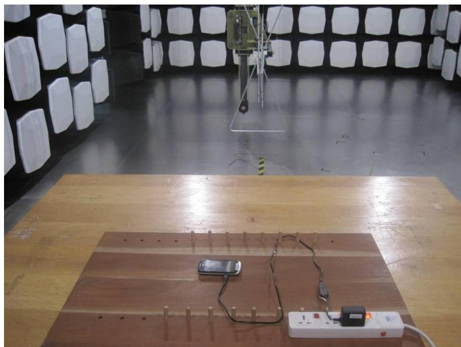
6. Part 15B Radiated emission(charger) above 1GHz
