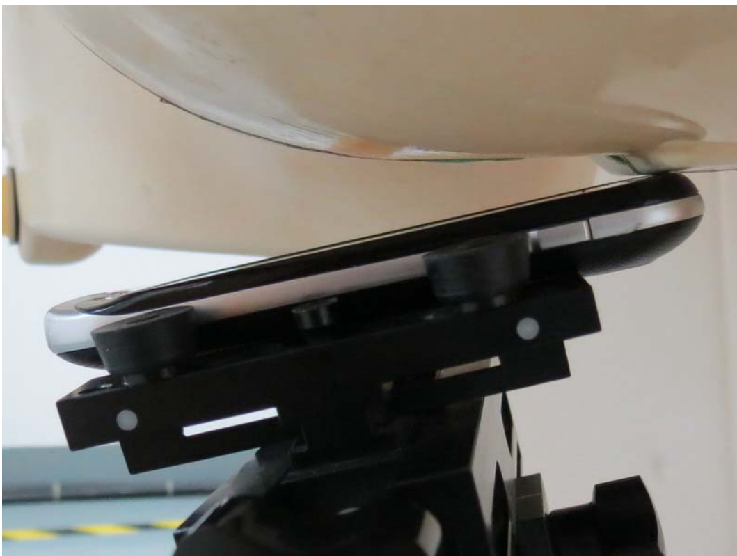
Picture 10: Left Hand Tilt 15 Degree Position
