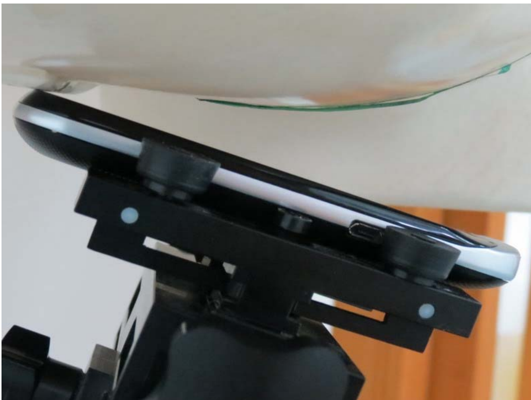
Picture 12: Right Hand Tilt 15 Degree Position
