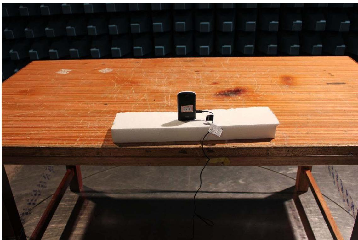
**FCC Part15C Radiated Emission below 1GHz****- Front**
