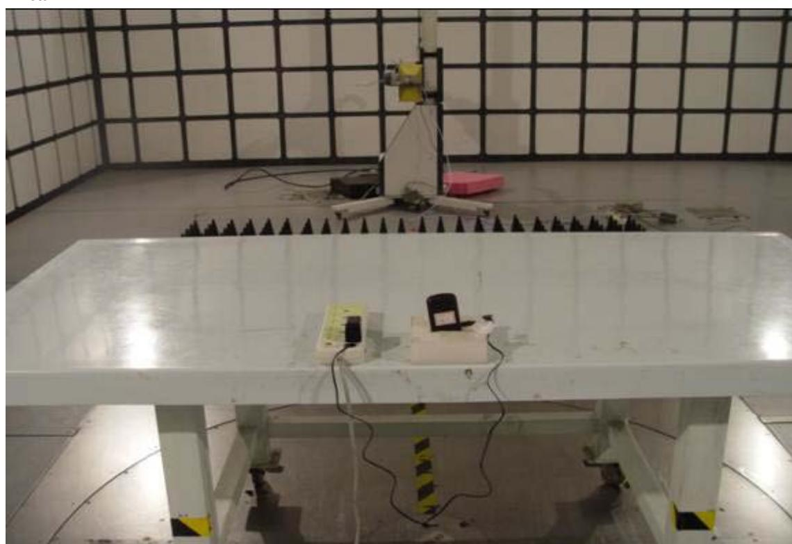
**AC Conducted Emission Test Setup**
