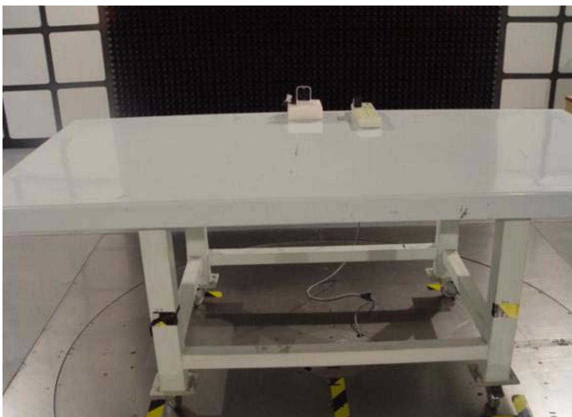
**FCC Part15C Radiated Emission above 1GHz****-Front**
