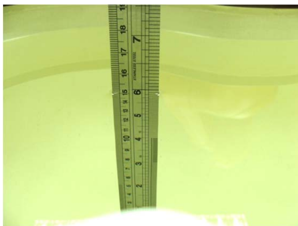
Fig 6.1 Photo of Liquid Height for Head SAR
