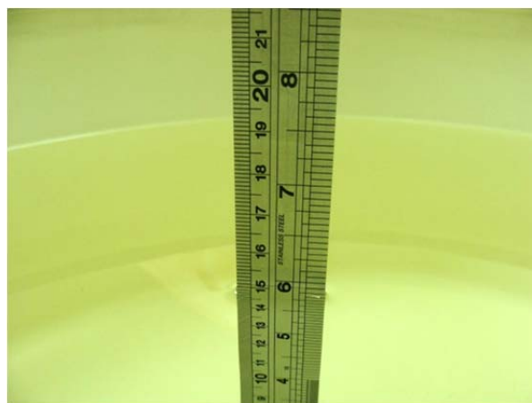
Fig 6.2 Photo of Liquid Height for Body SAR
