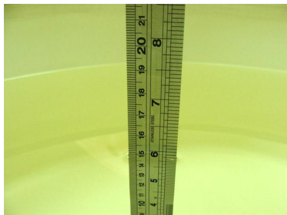
Fig 6.2 Photo of Liquid Height for Body SAR
