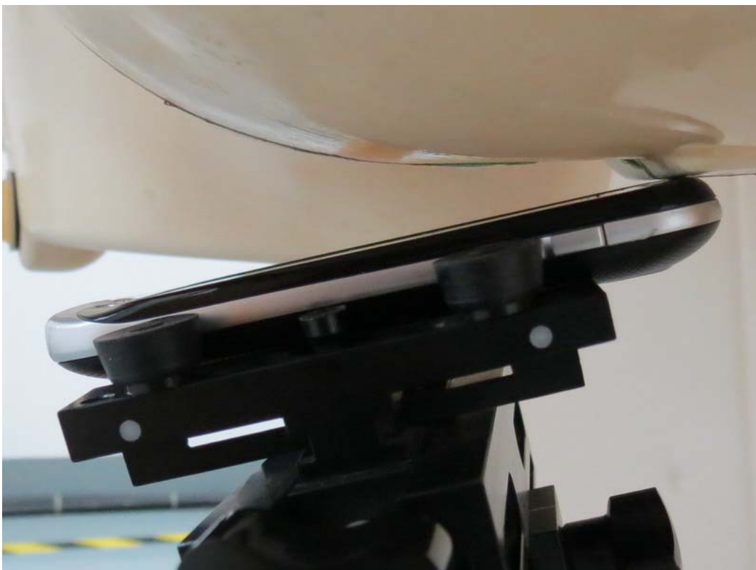
Picture 10: Left Hand Tilt 15 Degree Position
