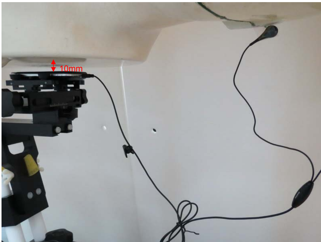
Picture 20: Front Side with earphone, the distance from handset to the bottom of the Phantom is 10mm
