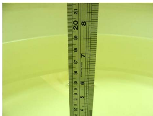
Fig 6.2 Photo of Liquid Height for Body SAR
