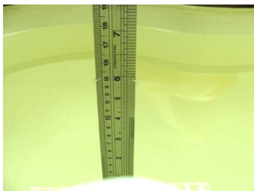
Fig 6.1 Photo of Liquid Height for Head SAR
